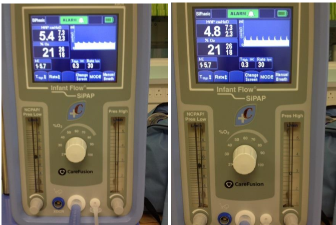
Picture 1 – Unlicensed Consumable. – waveform fails to achieve Biphasic breath for set iTIME.
